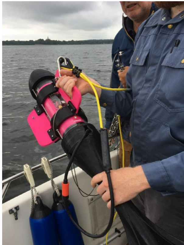
Figure 2: The picture shows the towbody before deployment. The towbody is easily handled manually, and it can be deployed from small boats. This allows local fishers to use the towbody without special equipment. Photo by Fletcher Thompson.
